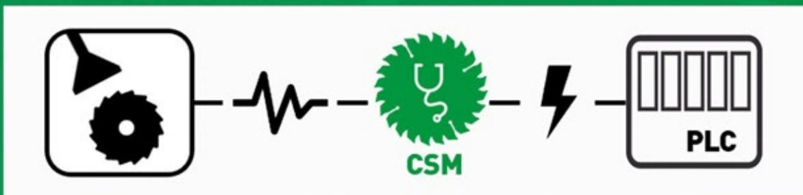
The systems include a highly sensitive microphone, an electronic part and the CSM software, which is integrated into the existing control software.
