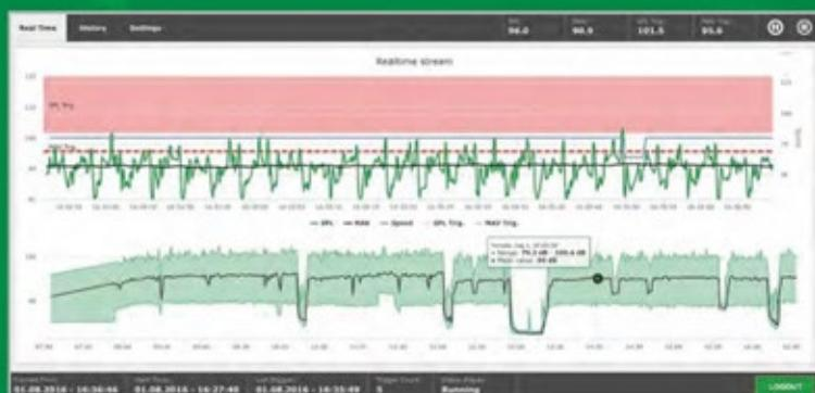
Sound level measurement curve SPL (top): At 16:35:59 the SPL exceeds the set limit (red area), the feed (blue line) is immediately slowed down briefly. This effectively prevents damage to the saw blades.
